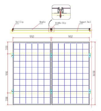
Mounting Drawing 1 (with clamping clips)
