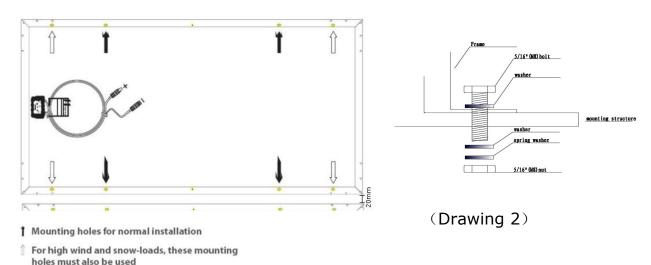
The frame of each module has 4 mounting holes (12mm\*9mm) used to secure the modules to supporting structure. The module frame must be attached to a supporting structure using M8 stainless steel hardware together with spring washers and flat washers in four places symmetrical on the Perlight Solar module. The applied torque is about 8 Newtonmeters.
